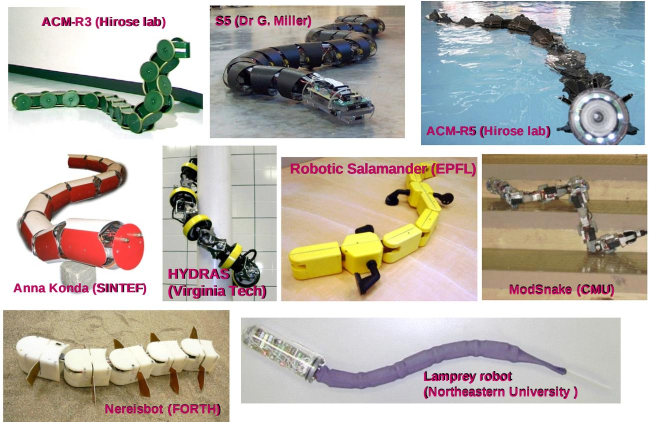
Figure 2: Hyper-redundant robotic locomotion systems.
