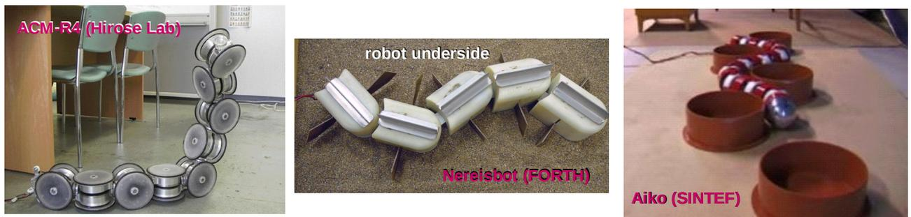
Figure 4: Interaction with the locomotion environment through passive wheels [HF04] (left), blade-like modules generating differential friction [ST09] (middle), and via push-point contacts [TLGP08] (right).
